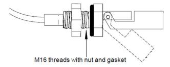
WIRING DIAGRAM Switch is closed when float is near stem Red wire L1 N.C. \_\_\_\_\_\_Red wire
