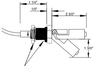
Gasket: As the nut is tightened on the thread, the gasket diameter will expand.
